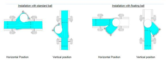
During the assembly of the ECON ball check valves, the following rules should be observed:
