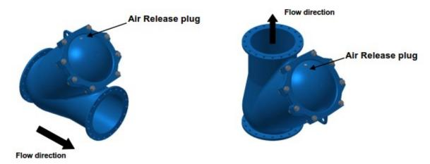
To eliminate the air proceed by unscrewing the plug in order to release the accumulated air until the fluid is coming out. The plug is auto blocked and cannot be unscrewed totally. If the plug is damaged or blocked, proceed disassembly of the bonnet as indicated in previous content. It is recommended to clean the plug when bonnet is disassembled for maintenance.
